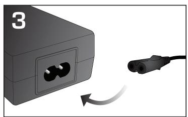
Plug the appropriate end of the power cable into the power adapter.
